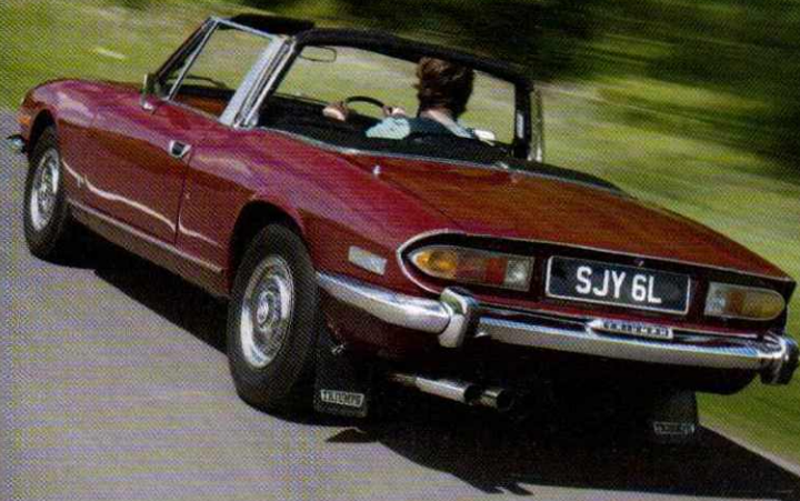
T-shaped roll-over bar robs the Stag of its pure convertible looks but aids rigidity
